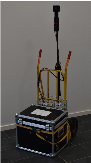
Figure 1: The equipment as used during the field measurements. The probe antenna is mounted on the pole on top, and the box contains the spectrum analyzer, laptop computer and battery power supply.
